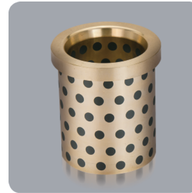
RFB 2102.70. 材料: 高力黄铜+ 固体润滑剂 Material: CuZn25Al5Mn3Fe3 + Graphite (500#SP) 推荐座孔 H6
